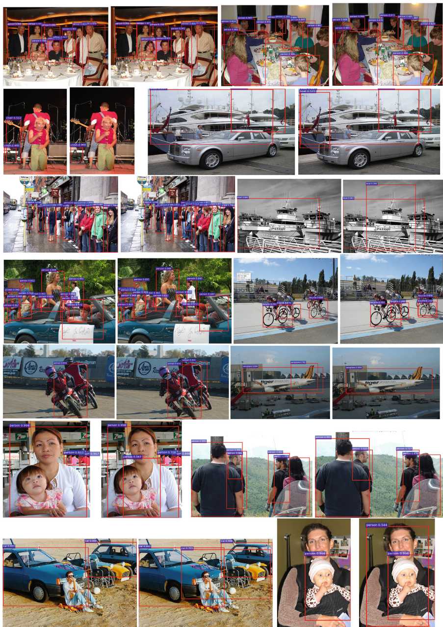
Fig. 3. Selected examples of object detection results on the PASCAL VOC 2007 test set using the Faster R-CNN system. The model is VGG-16 and the training data is 07 trainval. Left for NMS algorithm and right for Continuous Penalty-NMS1 algorithm.
