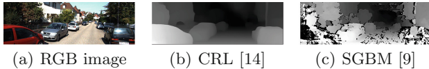
Fig. 5. Disparity maps from CRL [14] and SGBM [9]. Best viewed in color. (Color figure online)
