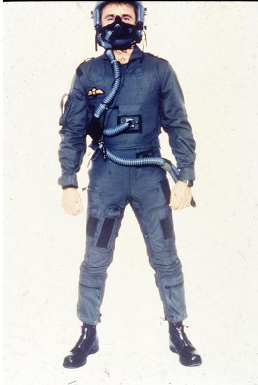
**Fig. 3** Representative Positive Pressure Breathing Ensemble. Picture shows the helmet/oronasal mask, thoracic jerkin, anti-G suit, and connectors/tubing. The breathing system is tied into the aircraft's life support breathing supply and regulator (blend of bottled O<sub>2</sub> and engine bleed air). Reproduced with permission from the Canadian Department of National Defence. The source is Defence R&D Canada
