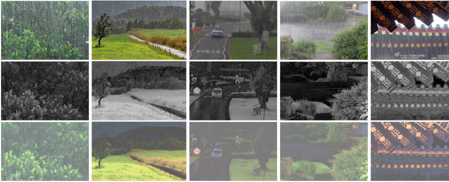
Fig. 2. Top: Images captured in rain scenes with rain streaks and rain accumulation. Middle: Residue channels of the corresponding rain images. Bottom: The colored residue images of the corresponding rain images. The rain streaks are significantly reduced in the residue channel and colored-residue images, though some regions become dark due to achromatic background and rain accumulation. Note, we increase the intensity of the dark regions for visualization purpose.
