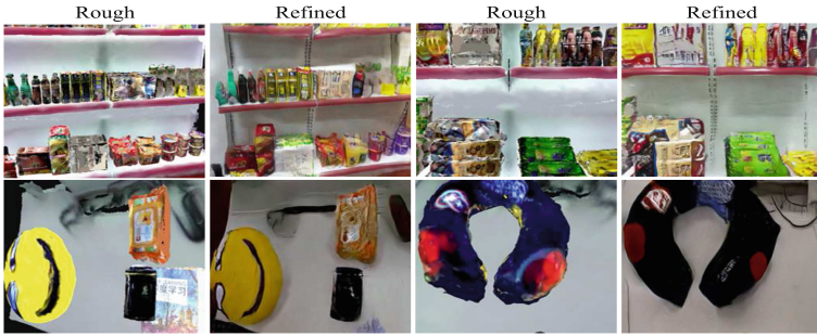
Fig. 7. Refinement of GAN. Refined column is the result of GeoGAN and rough column is the rendered image. Apparent improvement on lighting conditions and texture can be observed.
