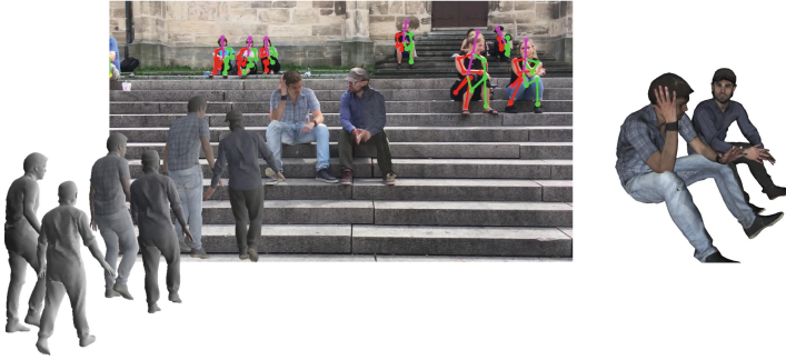
Fig. 1. We propose Video Inertial Poser (VIP), which enables accurate 3D human pose capture in natural environments. VIP combines video obtained from a hand-held smartphone camera with data coming from body-worn inertial measurement units (IMUs). With VIP we collected 3D Poses in the Wild , a new dataset of accurate 3D human poses in natural video, containing variations in person identity, activity and clothing.
