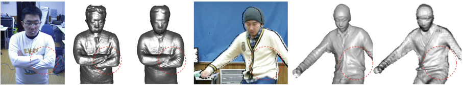
Fig. 9. Application on DynamicFusion (left) and DoubleFusion (right) using our enhanced depth stream. Left: color image, Middle: fused geometry using raw depth stream, Right: “instant” geometry using our refined depth stream.
