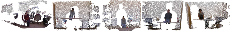
Fig. 2. CAD-120 Point Clouds. We evaluate NGM on the CAD-120 dataset, which contains RGB-D videos of everyday actions. We visualize single point cloud frames where each point is the 3-D projected (x_i, y_i, z_i) of the corresponding depth frame.
