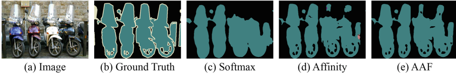
Fig. 1. We propose new pairwise pixel loss functions that capture the spatial structure of segmentation. Given an image (a), the task is to predict the ground-truth labeling (b). When a deep neural net is trained with conventional softmax cross-entropy loss on individual pixels, the predicted segmentation (c) is often based on visual appearance and oblivious of the spatial structure of each semantic class. Our work imposes an additional pairwise pixel label affinity loss (d), matching the label relations among neighbouring pixels between the prediction and the ground-truth. We also learn the neighbourhood size for each semantic class, and our adaptive affinity fields result (e) picks out both large bicycle shields and thin spokes of round wheels.
