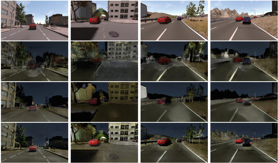
Fig. 2. SYNTHIA day-to-night transformation results - GANs trained with SYNTHIA: first row: SYNTHIA daytime testing images; second row: results of CycleGAN; 3rd row: results of UNIT; 4th row: results of AugGAN
