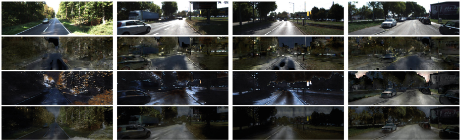
Fig. 4. KITTI day-to-night transformation results - GANs trained with SYNTHIA: first row: KITTI images; second row: result of CycleGAN; 3rd row: result of UNIT; 4th row: result of AugGAN.
