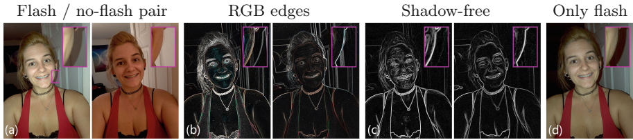
Fig. 4. For an unaligned flash and no-flash photograph pair (a), we compute the shadow-free edge representations (c) from the RGB image gradients (b). Inset shows the edge of the shadow in the flash image (b) disappearing in our representation (c). We estimate the alignment using the shadow-free representations and subtract the no-flash image from flash image after alignment to get the flash-only illumination (d).
