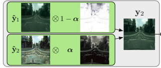
Fig. 4. Illustration of the linear combination in an adaptive fusion block. The fusion block applies the fusion weight map \alpha to find defects in the previous result \hat{y}_1 and correct it precisely using \hat{y}_2 to produce a refined output y_2 .
