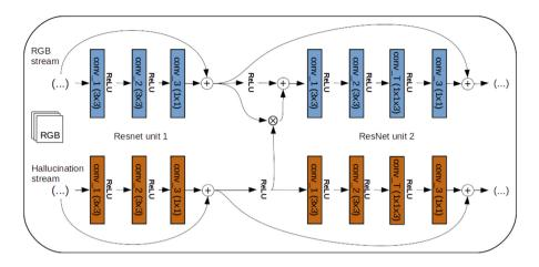
Fig. 2. Detail of the ResNet residual unit, showing the multiplicative connections and temporal convolutions [5]. In our architecture, the signal injection occurs before the  $2^{nd}$  residual unit of each of the four ResNet blocks.
