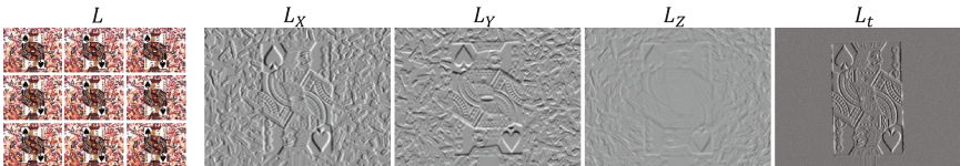
Fig. 4. Measured light field gradients. Light field for an example scene (a card moving in the X-Z plane in front of a static background) is shown as a 3 \times 3 subset of sub-aperture images (left). Light field gradients are only shown for the central sub-aperture. Zoom in for details.
