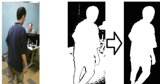
Fig. 2. The cropped color image (left), the grayscale depth representation \mathbf{D}_p^g (center) and the result after background subtraction (right) using the body index information \mathbf{B}_p from skeleton tracking.
