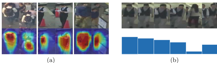
Fig. 1. Sample detections in the MOT16 dataset [35]. (a) Top row: image pairs with misalignments, missing parts, and occlusion. Bottom row: spatial attention maps for each image pair. (b) Top row: target trajectory containing noisy samples. Bottom row: temporal attention weights for corresponding images in the trajectory.
