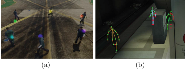
Fig. 4. (a) Visualization of TAFs for different parts: for clarity, we show a single joint TAF for each person where color encodes direction. (b) Pose prediction performed on JTA dataset which distinguish between visible and occluded joints
