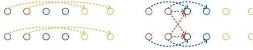
Fig. 5. Illustration for forcing local merge. We simulate the merging process with distance \{1, 2, 4\} and window size 2, we only show edges involved in this process. Pixels with identical colors are merged and we update the new weights for edges. The left graph shows that the new probability in distance \{2\} should only be averaged by the original weights from distance \{4\} in the same direction. However, the right graph shows the new probability for distance \{1\} should be an average of the edges from both distance \{1\} and \{2\} .
