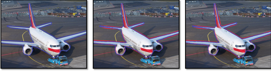
Fig. 2. Evolution of edge alignment during training (progression from left to right). Blue color indicates the aligned edge labels learned by SEAL, while red color indicates the original human annotation. Overlapping pixels between the aligned edge labels and the original annotation are color-coded to be blue. Note how the aligned edge labels gradually tightens around the airplane as training progresses. Best viewed in color. (Color figure online)
