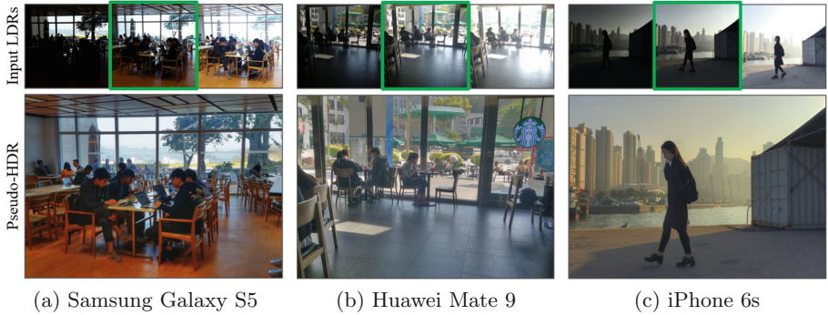
Fig. 10. HDR results without radiometric calibration. All examples are novel images taken using cellphones with different CRFs.
