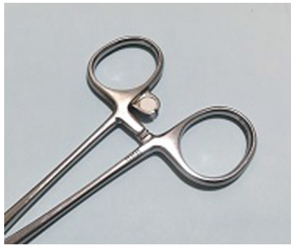
Fig. 1. Surgical instrument with RFID tag [3]
