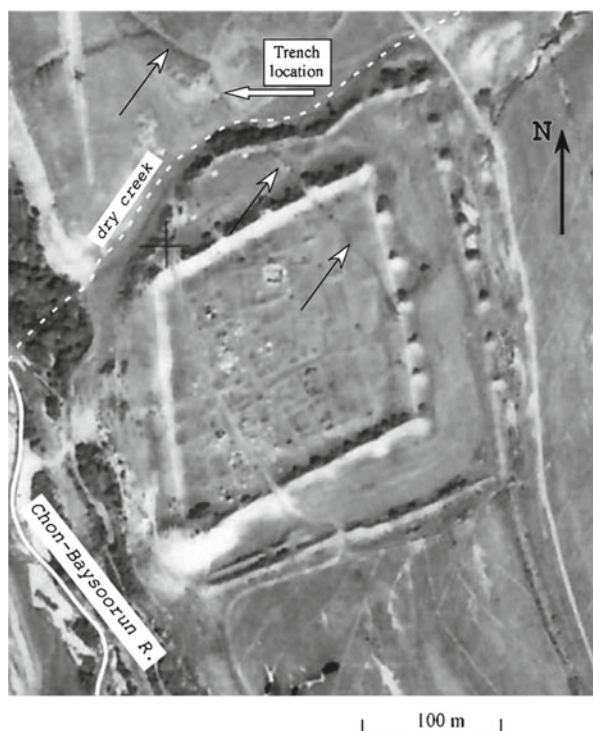
Fig. 7.4 Aerial image of the earthworks of Medieval Kamenka fortress north of Issyk Kul, Kyrgyzstan. The rhomb-shaped fortress, surrounded by towers, is cross-cut by an active fault (marked with arrows), which caused 4 m left-lateral displacement during the M 8.2 Kemin earthquake in 1911. Rammed earth walls survived with minor damage (Korjenkov et al. 2006a, Povolotskaya et al. 2006)
