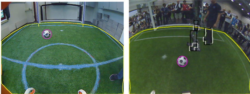
Fig. 4. Left: a captured image with detected ball (pink circle), field lines (light blue), field boundary (yellow lines), and goal post (dark blue lines). Right: visualisation of our obstacle detection. (Color figure online)
