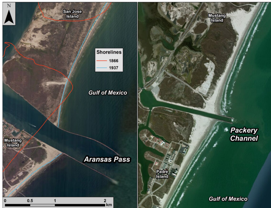
Figure 6.54. Patterns of deposition adjacent to the jetties at Aransas Pass and Packery Channel documenting variable transport directions. Shorelines from Miller et al. (2004). Image credit: ArcGIS World Imagery.
