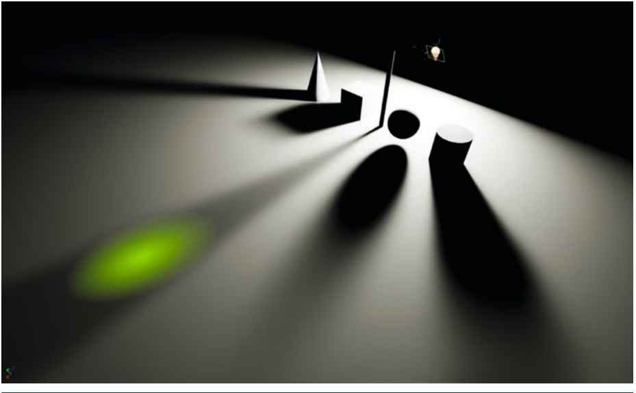
Figure 19-5. Visualization (in green) of a filter kernel used in our shadow denoiser. Notice how it is anisotropic and stretches along each penumbra's direction. (From Liu [7].)
