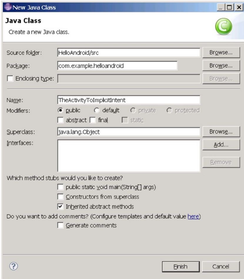
Figure 3-19. New class for the custom activity of the corresponding implicit intent
