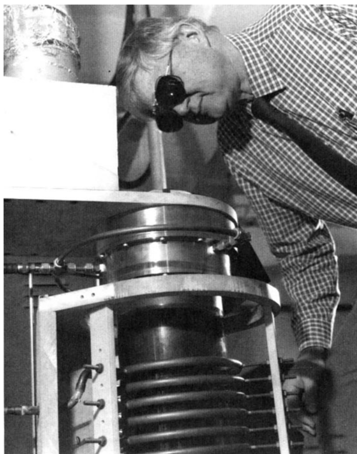
Fig. 2. Researcher Dan Barrett (Westinghouse Science & Technology Center) checks the hot (2400°C) crystal growth furnace that he designed for physical vapor transport growth of single crystals of silicon carbide.
