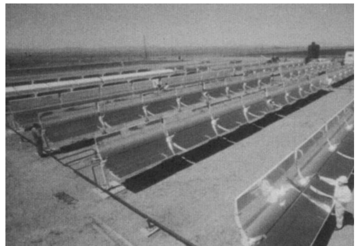
Fig. 10. (a) One configuration of an optical-type concentrator with axial absorber; (b) parabolic troughs under test for various uses, including irrigation pumping for croplands.
