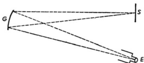
Fig. 2. Concave grating spectroscope: Slit, S; grating, G; eyepiece or plateholder, E.
