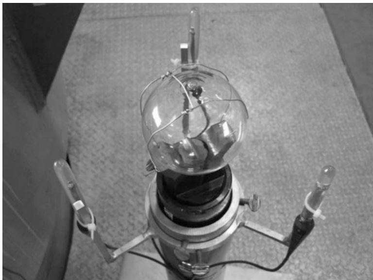
Fig. 6.6 Test stand with the glass sphere test specimen and the instrumentation installed (Turner 2007)
