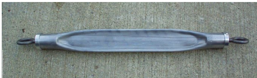
Fig. 6.18 Collapsed shape of the aluminum cylinder after the implosion experiment
