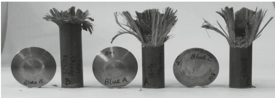
Fig. 8.5 Photograph showing failed specimens and corresponding striking masses accelerated by the detonation of 5, 9, and 13 g of PE4. Kakogiannis et al. (2009)
