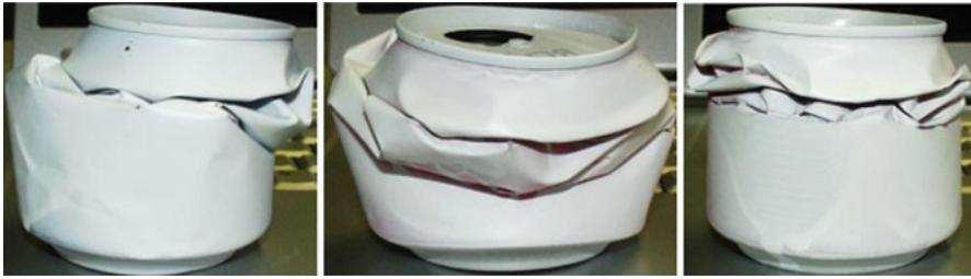
Fig. 8.11 Photograph showing crushed empty beverage cans as a result of the close-range free air blast (Palanivelu et al. 2011a)
