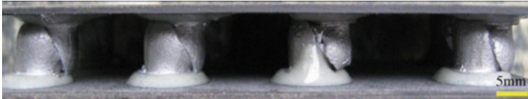
Fig. 8.23 Failure of hollow tubes under compressive load (Xiong et al. 2011)
