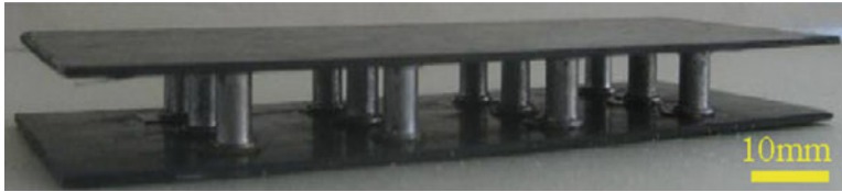
Fig. 8.22 Photograph showing a sandwich panel with hollow Al-Si alloy tube core (Xiong et al. 2011)
