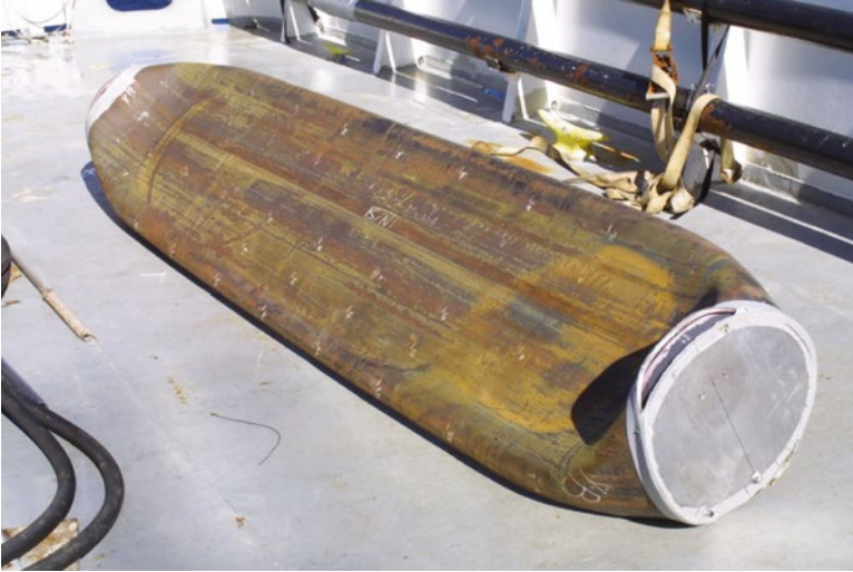
Fig. 6.24 Collapsed shape of the 45.7 cm (18 in.) steel cylinder after the at-sea implosion test
