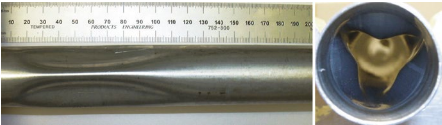
Fig. 7.11 Post-collapse photographs of tube following the test which generated the data shown in Fig. 7.10 and illustrating buckling in mode 3. Tube is 6061-T6 aluminum with mean radius a = 15 mm and a/h = 17.4
