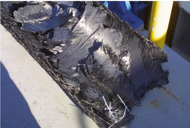
Fig. 6.25 Collapsed shape of the 45.7 cm (18 in.) GRP composite cylinder after at-sea implosion testing
