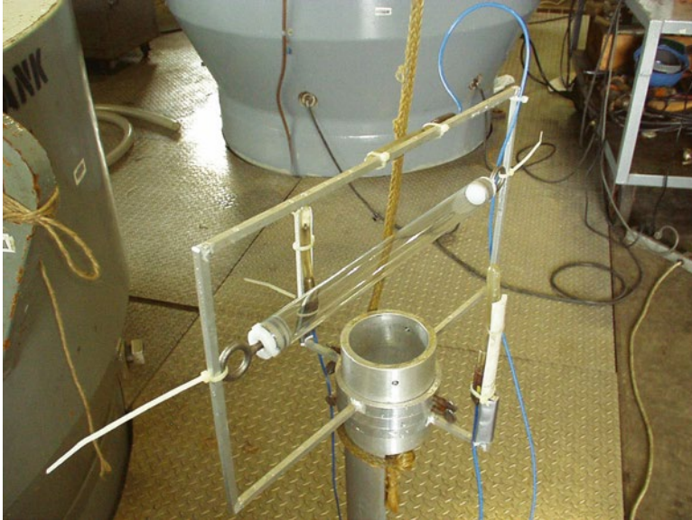
Fig. 6.21 Test stand after glass cylinder implosion experiment (Turner 2004)
