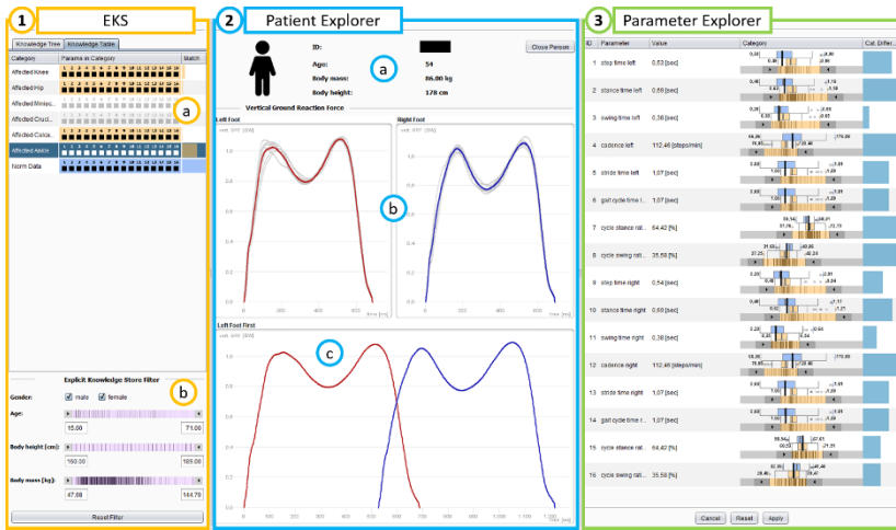
Fig. A.123: KAVAGait's user interface, which combines three main components: (1) the explicit knowledge store (EKS) capturing an overview of the stored gait patterns, (2) the patient explorer combining patient's information and different visualizations of the ground reaction force, and (3) the parameter explore visualizing the 16 calculated spatio-temporal parameters of the patient to be explored in connection with various statistical measures. © Wagner et al. (2019).
