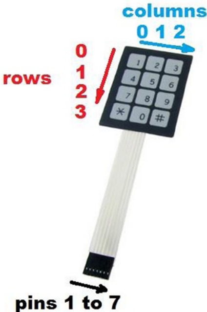
Figure 9-4. Keypad disposition of pins and identification of rows and columns
