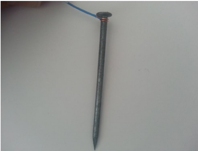
Figure 8-4. Wrapping the wire around the nail's head
