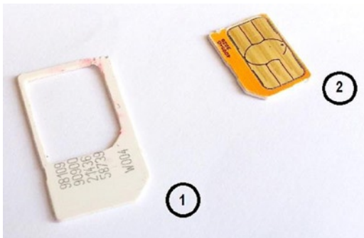
Figure 12-3. Nano-to-micro-SIM adaptor (1) and nano-SIM card (2)
