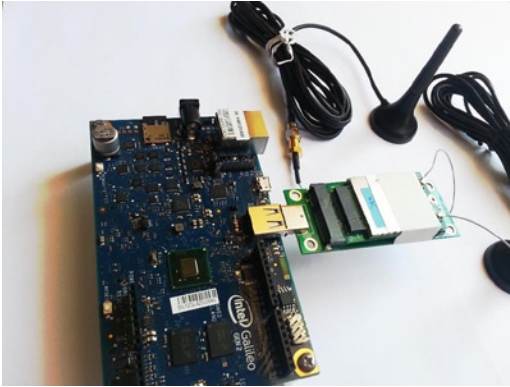
Figure 12-13. Connecting the devices to Intel Galileo Gen 2
