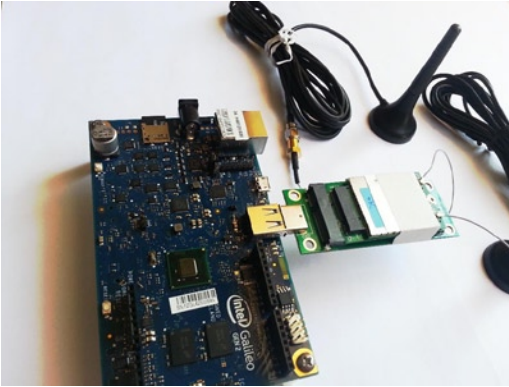
Figure 12-13. Connecting the devices to Intel Galileo Gen 2
