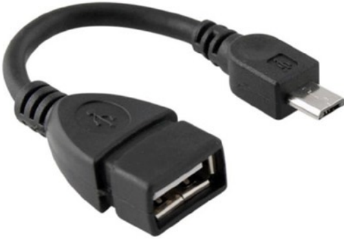
Figure 5-20. Micro USB to USB 2.0 OTG adapter
