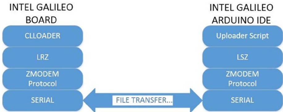
Figure 5-21. The regular file transfer mechanism
