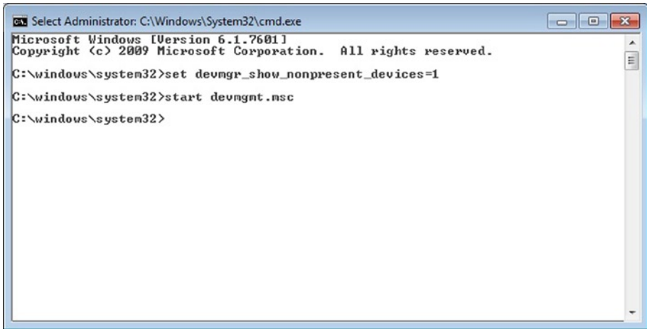
Figure 3-19. Starting the Device Manager via the Command Prompt
