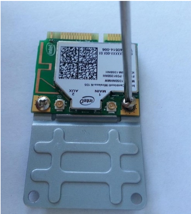
Figure 5-1. Connecting the bracket to the WiFi card
