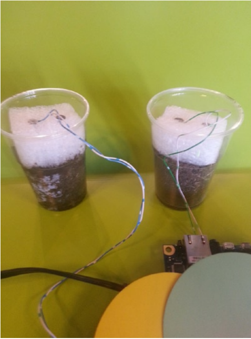
Figure 8-12. The sensors in the cups
