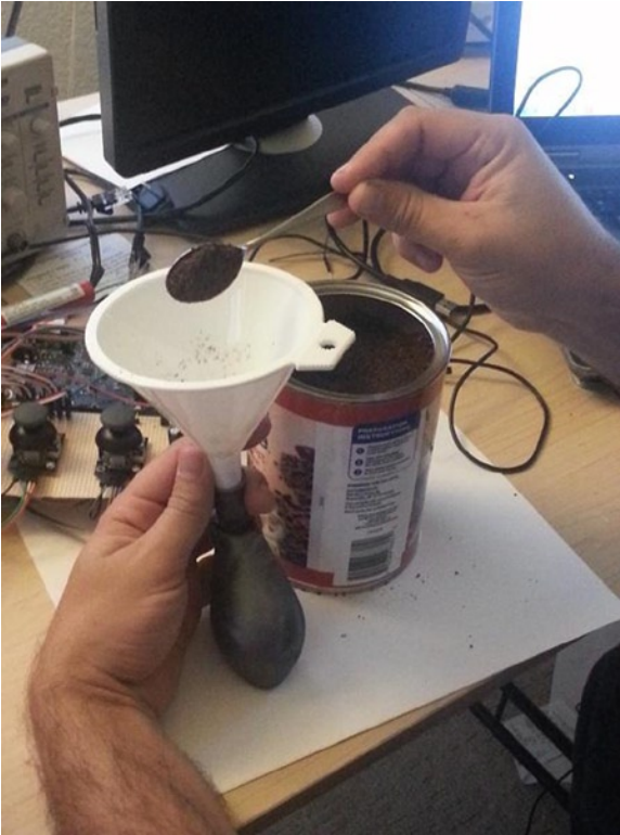
Figure 11-51. Filling the gripper with ground coffee
