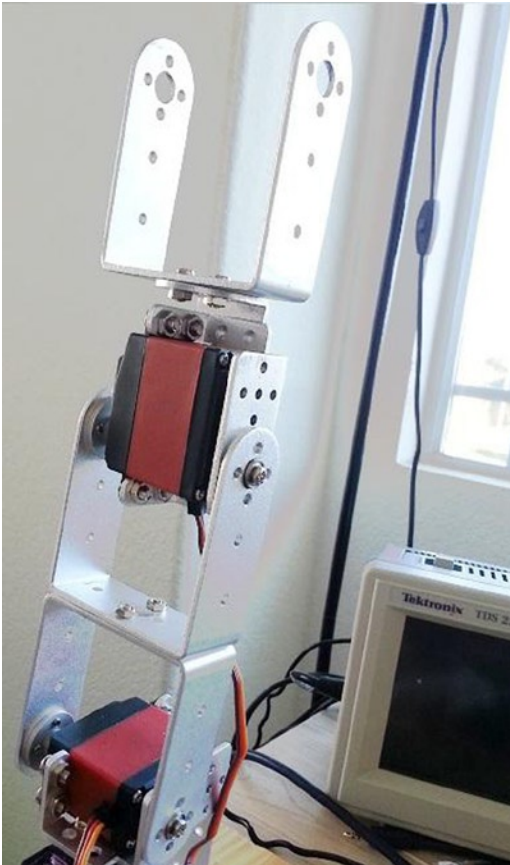
Figure 11-28. Elbow connected to the arm
