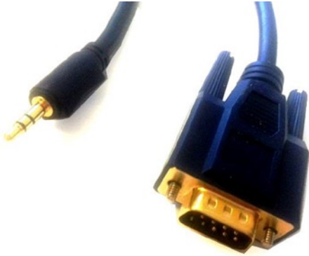
Figure 1-14. Cable with a DB9 male connector to a 3.5mm jack
