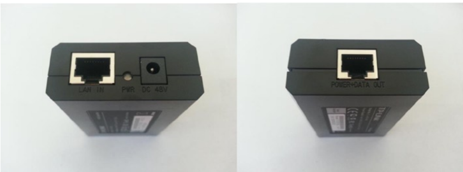
Figure 10-6. The LAN IN (left) and POWER+DATA OUT (right) ports
