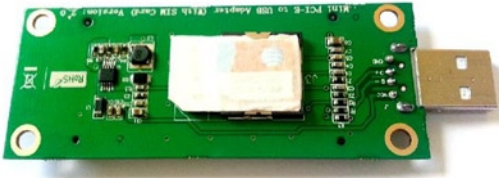
Figure 12-5. Connecting the SIM card
