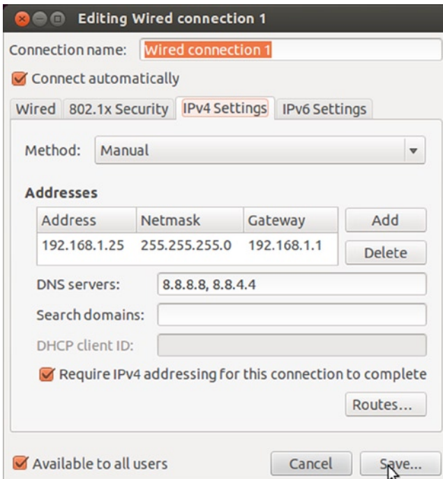
Figure 5-14. IPv4 properties with static IP only
