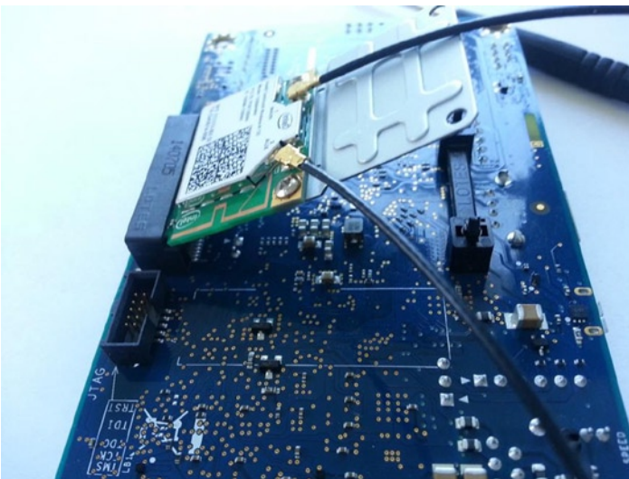
Figure 5-3. Connecting the WiFi card and bracket at an angle
