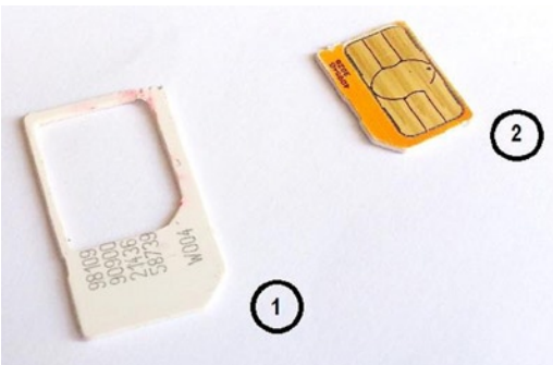
Figure 12-3. Nano-to-micro-SIM adaptor (1) and nano-SIM card (2)
