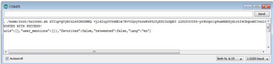
Figure 6-15. Debug messages from the serial console after a tweet
