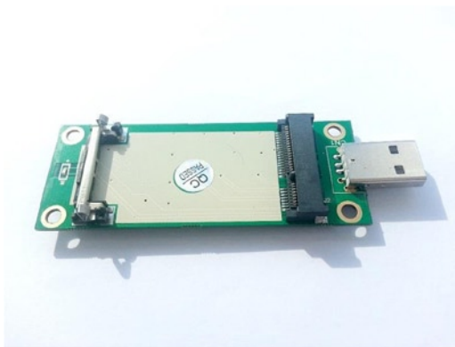
Figure 12-1. mPCIe to OTG-USB adaptor, top view
