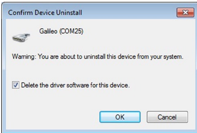
Figure 3-23. Deleting the hidden COM port and driver
