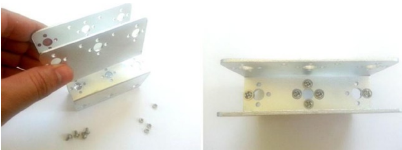
Figure 11-13. Connecting two U-shapes for the base
