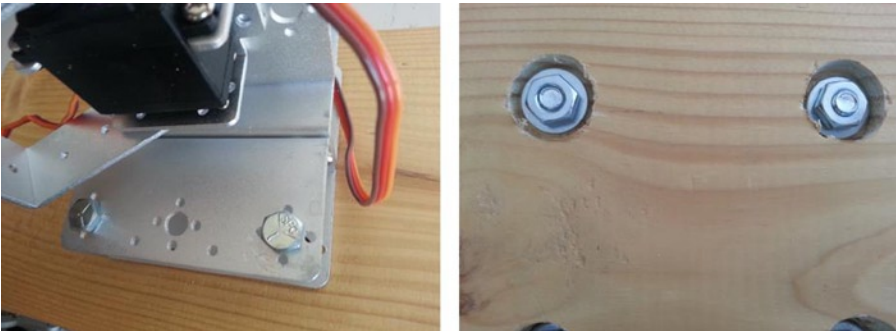
Figure 11-37. Top view of base with screws (left); bottom view with nuts (right)
