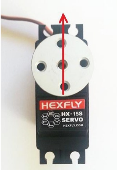
Figure 11-12. Servo wheel placed at 90 degrees
