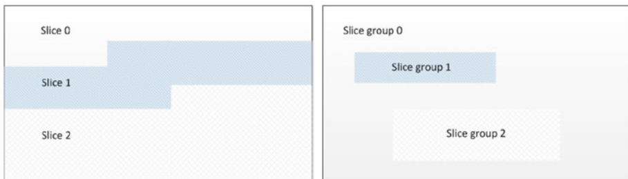
Figure 5-2. Partitioning of a video frame into slices and slice groups
