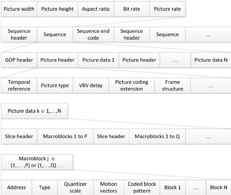
Figure 3-7. Structure of MPEG-2 video bitstream syntax
