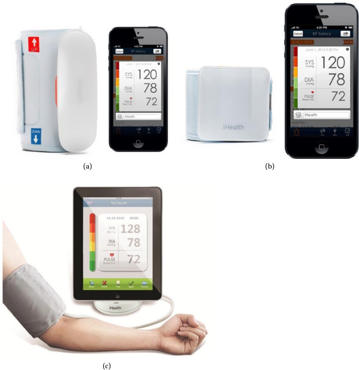
Figure 9-6. Blood pressure cuffs with smartphone and tablet connectivity (image used with permission from iHealth Labs)
