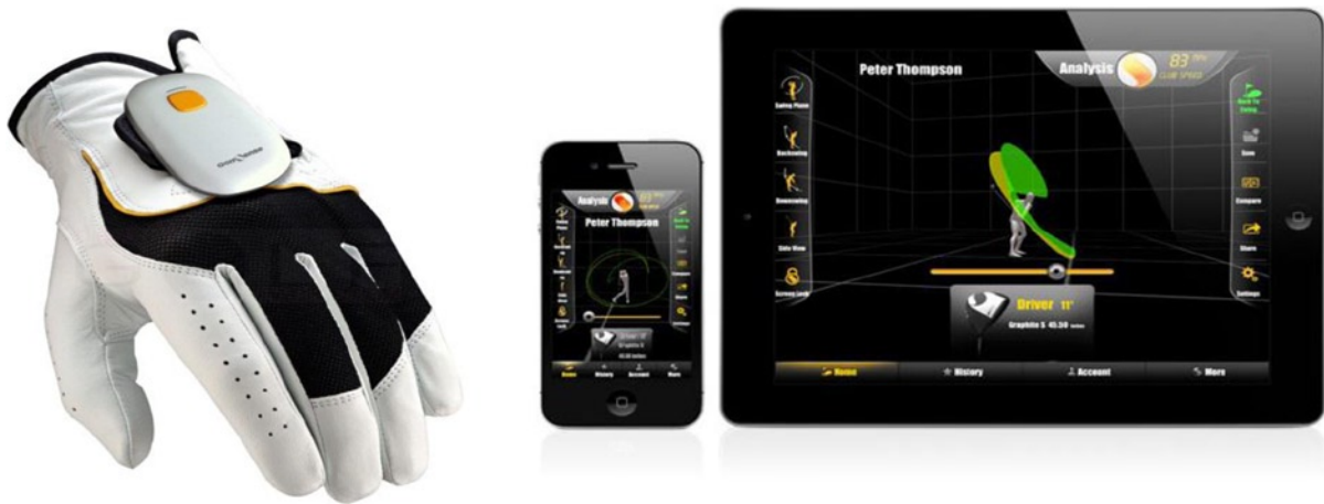
Figure 10-5. The Golfsense inertial sensor for golf swing analysis (image used with permission from Golfsense)
