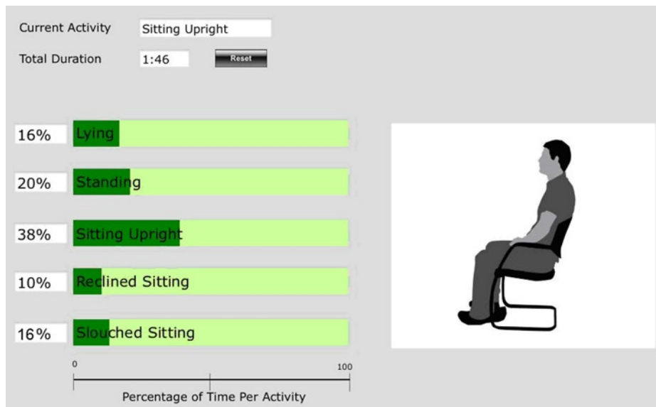
Figure 10-9. Posture monitoring and classification using inertial sensors
