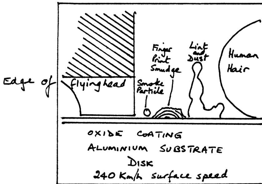
Typical Causes of electronic system & equipment failure
