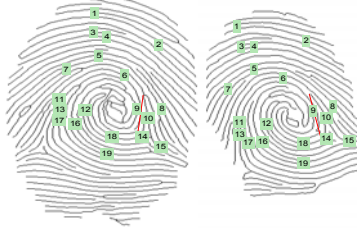
Fig. 6 Matched minutia pairs in two images of the same fingerprint; the red lines in the picture denotes optimal reference bi-minutia bar; the blue numbers in the picture represent corresponding orders of matched minutia pairs. The left is the ridge image of 1_3.gif in DB1_A of FVC2004, while the right is 1_6.gif.
