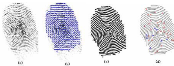
Fig. 1 Fingerprint preprocessing.(a)An original fingerprint in DB1_Aof FVC2004,(b)its block orientation field,(c)enhanced image,(d) thinned image of fingerprint image
