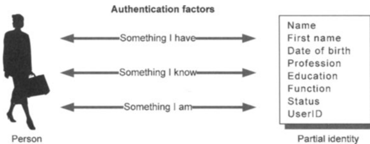
Fig. 4. The verification of the correct assignment of a digital (partial) identity to the physical (or legal) person is a weak point in all security systems. There are three different concepts (called factors) to establish a link between a physical person and its digital identity.
