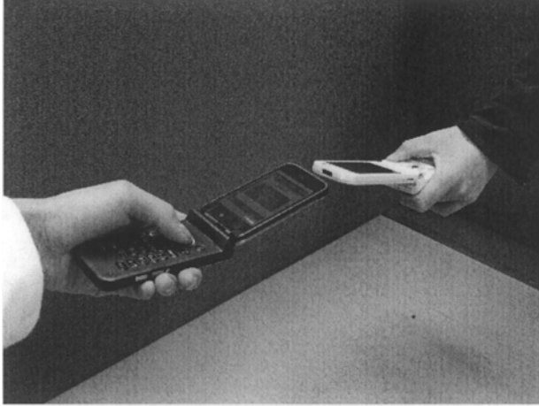
Fig. 3. An infrared communication between mobile phones
