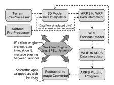
**Fig. 2.** Typical weather forecasting workflow in LEAD. It goes through stages of ingesting and preprocessing observational data, assimilating it into a 3D grid, running the prediction model on it, and disseminating the forecast as graphics and animations. Each box is a service and their execution is orchestrated by the workflow engine in the center.
