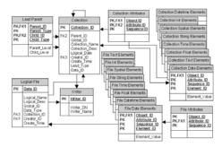
**Fig. 3.** Simplified relational schema of the myLEAD database. The organizational details (experiments, projects, etc.) and application attributes are coded in the data and not in the schema. This gives the catalog independence from the scientific domain.
