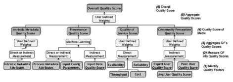
Fig. 6. Model to evaluate quality score of data product using various metrics applied to metadata attributes based on user-defined quality constraints. At the bottom are the attributes that affect the data's quality, and they are aggregated, using various metrics and user-defined constraints, to the overall quality score for the data at the top.
