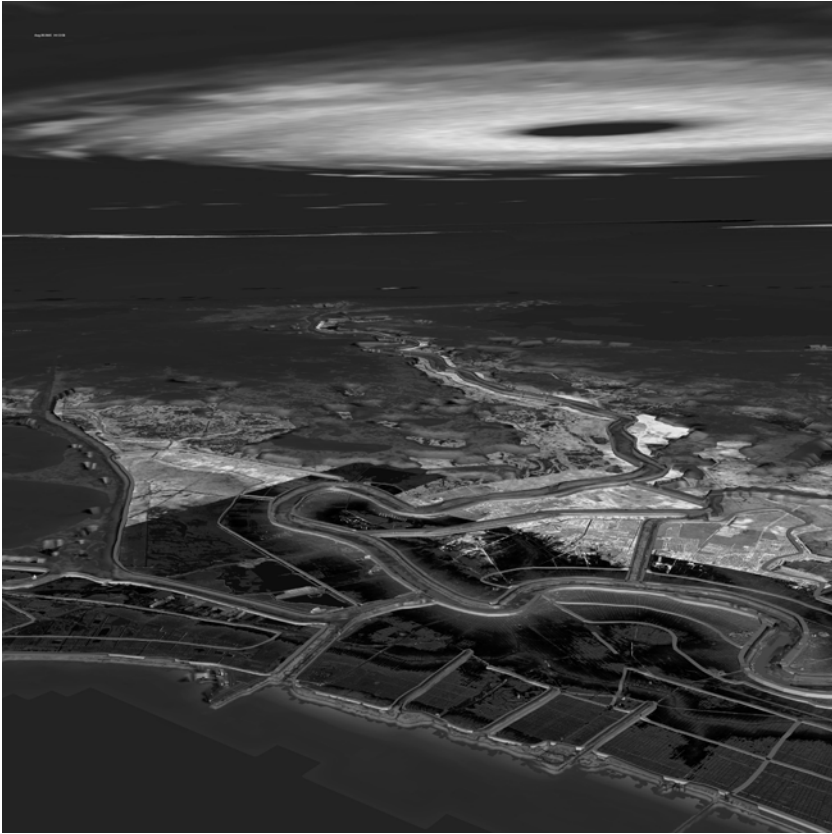
Fig. 8. Combined visualization of Hurricane Katrina approaching New Orleans, showing the water surge as predicted by the ADCIRC simulation model, cloud density as observed in infrared by the GOES-12 satellite, terrain height information obtained from high-resolution LIDAR measurements (green: above sea level, magenta: below sea level, blue: sea level) with the levee information of the ADCIRC model, overlaid on aerial photography and GIS terrain information. [Image credits: CCT Scientific Visualization group, Amanda Long, Werner Bengler, Ana Buleu, Shalini Venkataraman, Steve Beck].
