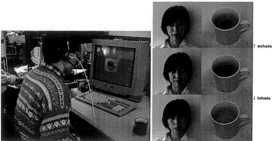
Figure 4. Manipulating interactive movies: For example, images of coffee in the cup or images of a human face thumb through according to the breath operation.
