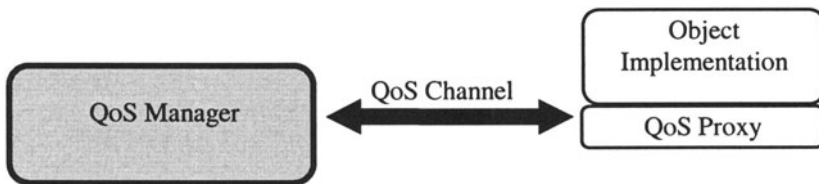
Figure 3. Role of QoS Channel between QoS Manager and QoS Proxy.
