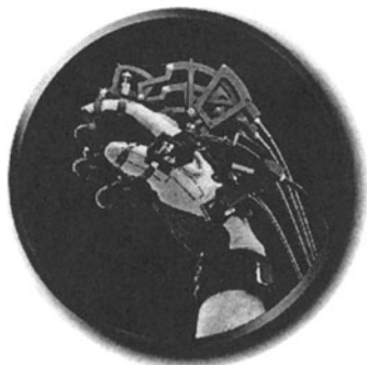
Figure 3: Haptic Feedback Device [1] built in the Glove Box and hidden from the user
