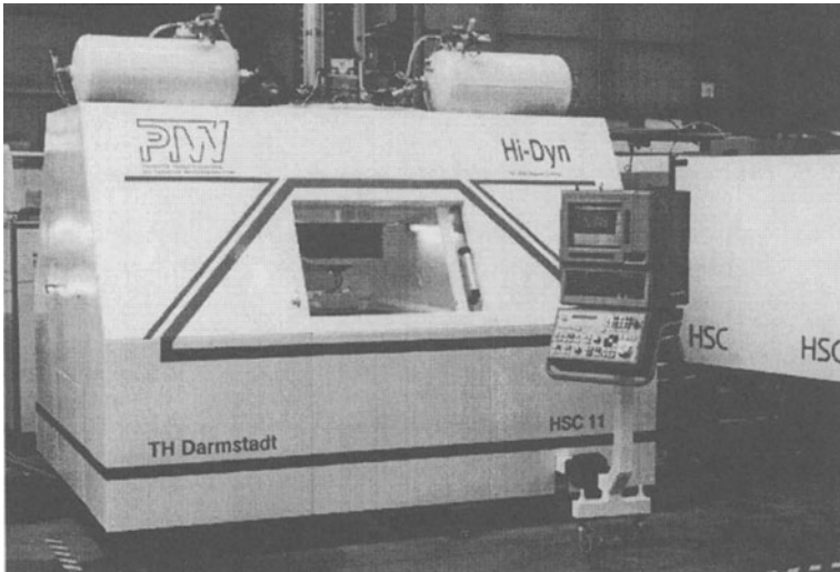
Figure 11. Highly dynamic 3-axis milling machine with linear feed drives
