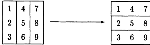
Figure 5 Two-dimensional transposition operation
