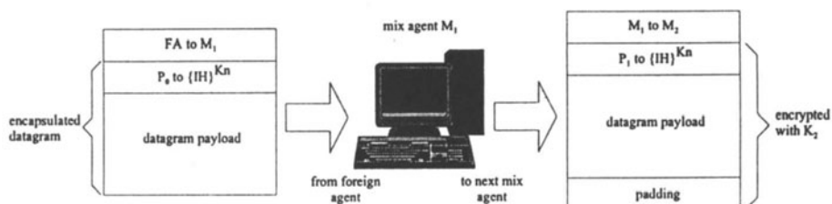
Figure 2 Tunneling in the Mixed Mobile IP
