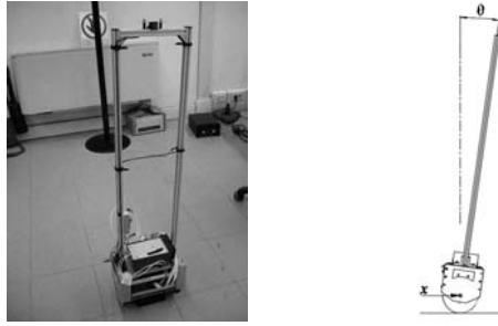
Fig. 1 The MWP robot Tilty and its degrees of freedom
