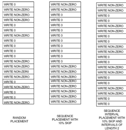
Fig. 3 Example of Different placement of zero-writes in our experiments (50% zero-writes) for 20 register-writes
