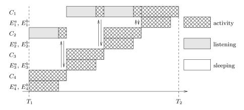
**Fig. 5.** The scheduled activities period starts at  $T_1$  and ends at  $T_2$ . According to the content of the beacon, star of  $C_4$  is the first to be active. At the same time, coordinator  $C_2$  is listening and waiting for  $C_4$  to finish communicating with its children and to initiate a parent-child communication. The same procedure applies to the other stars.
