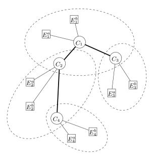
**Fig. 3.** A cluster-tree is built on a small topology, with  $C_1$  as a PAN coordinator.  $C_i$  represents a coordinator and  $E_i^x$  represents an end-device associated with coordinator  $C_i$ . Every coordinator constitutes a cluster with its children devices. For example, the cluster of coordinator  $C_2$  is formed by  $\{C_2, C_4, E_2^a, E_2^b\}$  and the cluster of coordinator  $C_3$  is formed by  $\{C_3, E_3^a, E_3^b\}$ .
