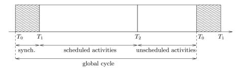
Fig. 1. MaCARI divides the time into three periods: a synchronization period between  $T_0$  and  $T_1$ ; a scheduled activities period from  $T_1$  to  $T_2$ ; an unscheduled activities period between  $T_2$  and the next  $T_0$ . The first two periods constitute the tree-based activities. The unscheduled activities are non tree-based activities and can be used for any routing protocol.
